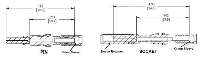
Note: After Polishing Sockets, slide the Split Alignment Sleeve over the Fiber Optic Termini and then slide the Sleeve Retainer over the Split Alignment Sleeve to the base of the Fiber Optic Termini. Apply Vibra-Tite VC-3 Threadmate on the threads per manufacturer's instructions. Screw the Sleeve Retainer onto the thread of the Fiber Optic Termini. Torque using the Sleeve Retainer Torque Tool PT-589 to the torque values in the torque table above.
