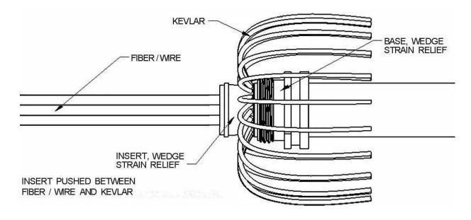
Cut Kevlar flush with top of wedge. Screw on Cap of Wedge Strain Relief. Torque to tighten using values from Torque Table above.
