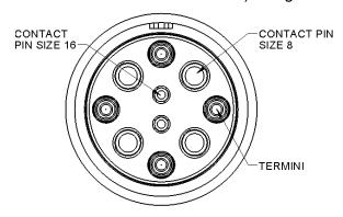
When populating using APC Fiber Optic Termini, align the key on the Fiber Optic Termini with keyway in the Insert.
