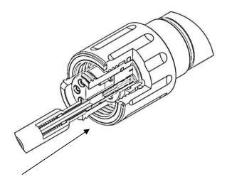
**For MT Insert** – Use MT Termini Insertion / Removal Tool PT-480 and slip Spring Push onto the prongs on the "insert" side of the tool and push MT Ferrule into the back cavity of the MT Insert. MT Ferrule should snap into place.
