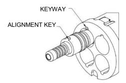
**For Hermaphroditic Insert** – Push in Fiber Optic Termini / Contact Pin and Sockets through back of Insert using appropriate Insertion (Tool PT-117 or PT-596). See configuration example below.
